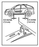
3. Near each wheel, there is a notch in the vehicle's body. Position the jack and raise the jack head until it fits firmly into the notch in the vehicle's frame nearest the flat tire. *Notice:* If you use a jack to raise the vehicle without positioning it correctly, you could damage your vehicle. When raising your vehicle on a jack, avoid contact with the rear axle control arms.
